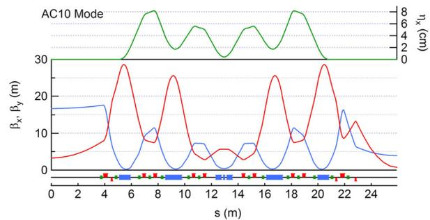
Figure 3: Lattice functions for Sirius half-superperiod in the AC10 mode.
