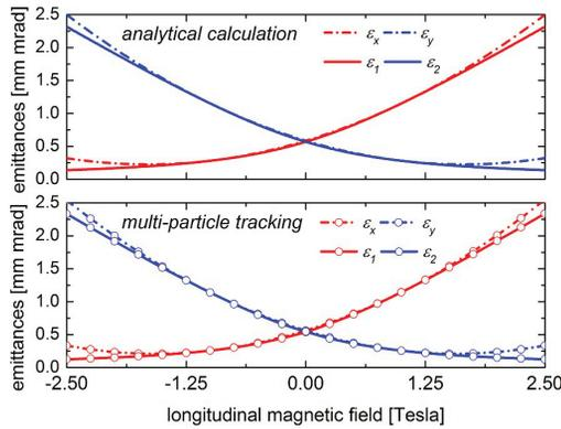
Figure 3: Eigen-emittances and rms emittances calculated by analytical method and by multi-particle tracking through the EMTEX beam line.
