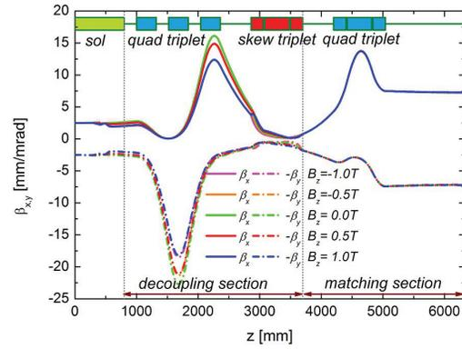
Figure 4: Horizontal and vertical beta-functions of the beam along the EMTEX beam line for different solenoid field strengths.
