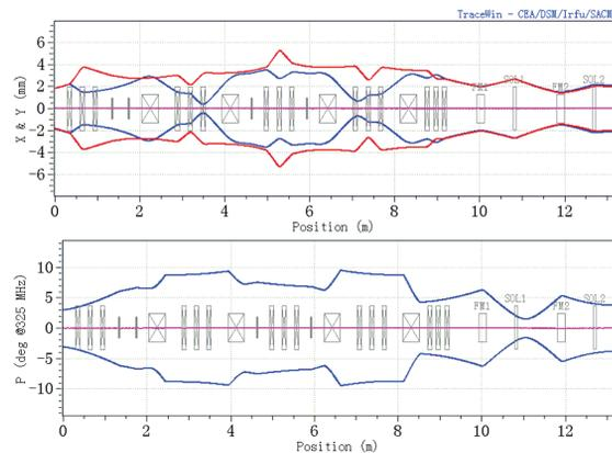
Figure 3: The rms beam size at  $x$  and  $y$  planes (upper plot) and the rms bunch length (lower plot).
