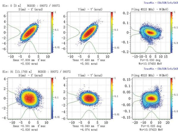
Figure 4: Particle distributions in phase spaces at MEBT2 entrance (upper plots) and exit (lower plots).
