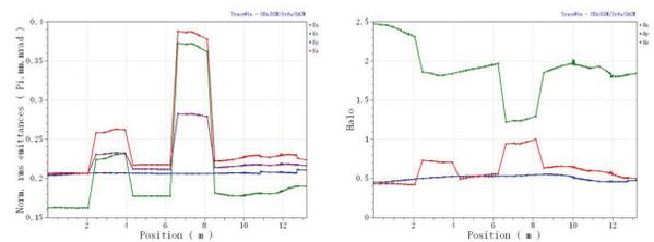
Figure 5: The rms beam emittance and halo parameters evolution along MEBT2 line.
