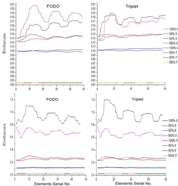
Figure 2: Beam emittance (cm mrad) evolutions in FODO and triplet cells with different initial distribution uniform (upper), real (lower).
