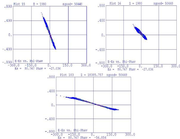
Figure 4: Longitudinal phase plots at debuncher entrance (upper L), debuncher exit (upper R) and RCS injection point (lower).
