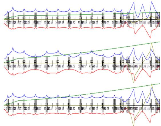
Figure 1: Comparison of LRBT beam envelopes and dispersion functions by TRACE 3D: without space charge (upper), mismatching (middle), re-match (lower).
