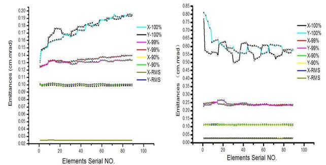
Figure 3: Beam emittance evolutions in LRBT after lattice optimization with different initial distributions: Uniform (left), real (right).
