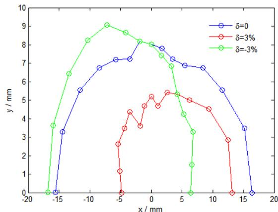
Figure 2: Dynamic aperture at the injection point of the new optics in the SSRF storage ring.
