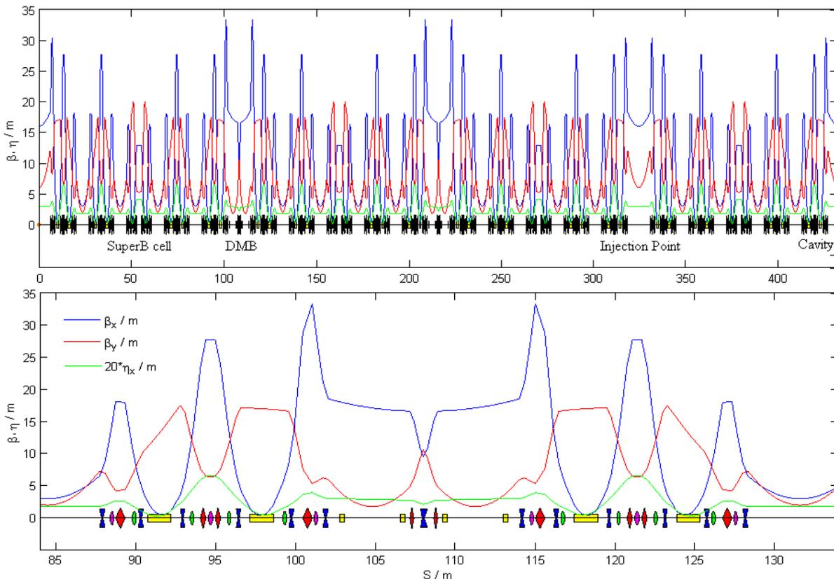
Figure 1: Linear optics along the SSRF storage ring and its double-mini- $\beta_y$  optics (DMB: Double-Mini-Betay).
