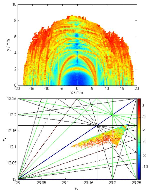
Figure 3: Dynamic aperture and frequency maps of on-momentum particle in the SSRF storage ring.
