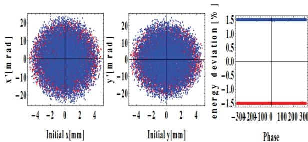
Figure 3: Beam distributions at ECR extraction.
