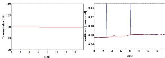
Figure 10: Beam transmission (left) and beam emittance growth (right) in the LEBT.
