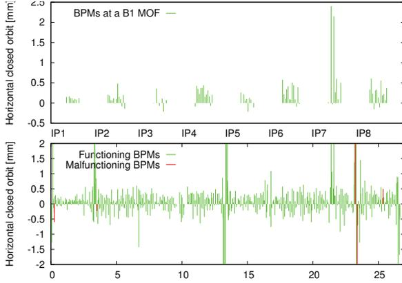
Figure 1: Beam 1 horizontal orbit logged at 02:19:54 during the *Octupole instability threshold MD*. Functioning BPMs are shown in green, others in red. The lower plot shows measured orbit at all BPMs. The upper plot shows the orbit measured at BPMs immediately preceding Beam 1 MOF.
