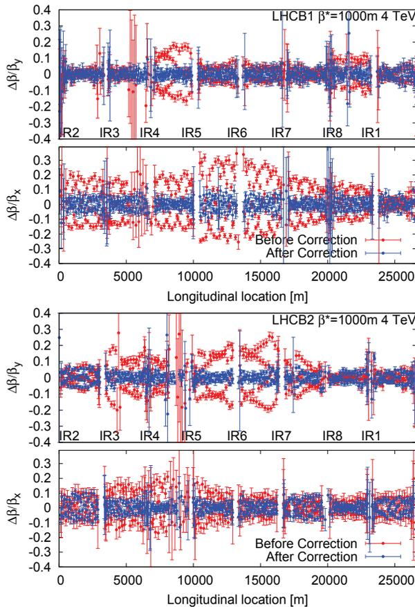
Figure 3: Measured  $\beta$ -beat at  $\beta^* = 1000\text{m}$ . Beam 1 is shown at the top and Beam 2 at the bottom.
