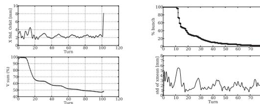
Figure 2: (a) shows the standard deviation of the horizontal BPM measurement and the charge reduction for an experiment in EMMA. (b) shows the same parameters for a bunch simulated in pyZgoubi with a magnetic model and bunch distribution approximately the same as the experiment. The beam is placed in a synchrotron bucket with 0.5 MV/turn acceleration.
