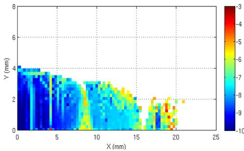
Figure 5: DA calculated using residual kickmap of VP mode (ID+shims) + 5mm apertures in one of 5mm gap in-vac ID.
