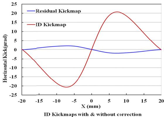
Figure 2: Horizontal kicks versus horizontal position with and without active shim.
