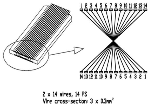
Figure 1: Shim wires set up.
