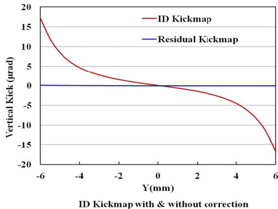
Figure 3: Vertical kicks versus vertical position with and without active shim.
