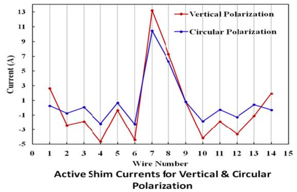
Figure 4: The current values of shim wires which produced optimal correction in VP and CP mode.
