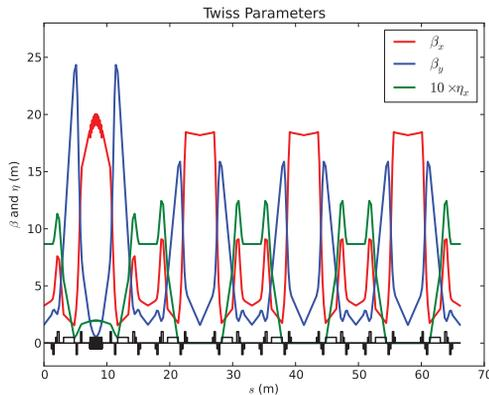
Figure 1: The rematched lattice of HLS-II storage ring.
