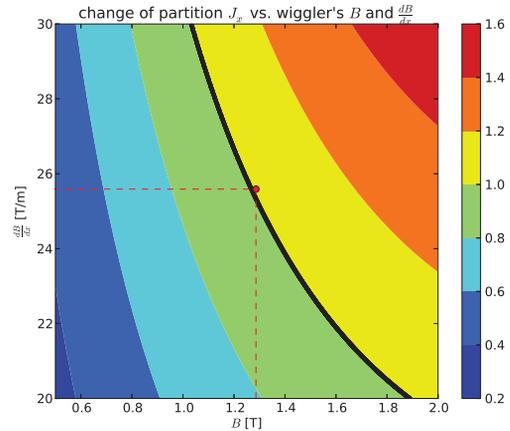
Figure 2: Contour of  $\Delta J_x$  changes with wiggler's field  $B$  and gradient  $\frac{dB}{dx}$  based on Eq. (4) and Eq. (5). The black line represents combinations of wiggler's field and gradient to achieve  $D = -1$ , i.e.  $J_x = 2$ . The red circle represents the Robinson wiggler's parameters we choose for our proof-of-principle study.
