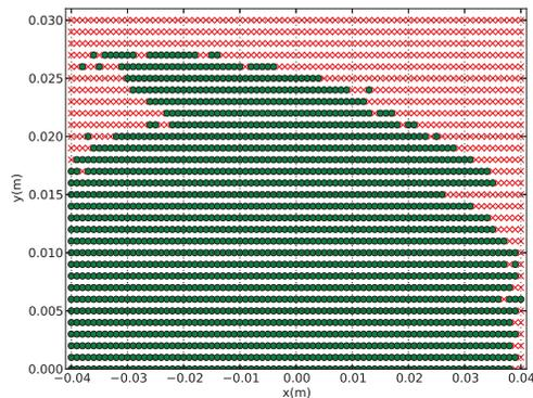
Figure 4: The dynamic aperture of the HLS-II storage ring with a perfect Robinson wiggler. The tracking starts from the center of the straight section. The green circles and red crosses represent the initial conditions of particles. With these initial conditions, the green circles mean the particles survive after 1024 turns, and the red crosses indicate the particles are lost before that.
