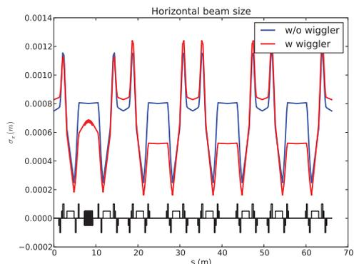
Figure 3: Horizontal beam sizes w/o Robinson wiggler. Comparing with the beam size of the bare lattice (shown in blue), a Robinson wiggler can decrease beam size significantly (up to 40%) in the non-dispersion straights, decreases slightly in the dipoles, and increases less than 10% in the dispersive straights as shown in red.
