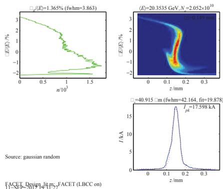
Figure 8: Simulated bunch profile from LiTrack in the FACET experimental area for 6mm long NDR bunches.
