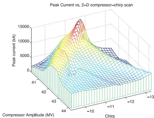
Figure 7: Simulated peak current from LiTrack in the FACET experimental area for 8mm long NDR bunches as a function of NRTL compressor amplitude and “staggered\_chirp” setting.
