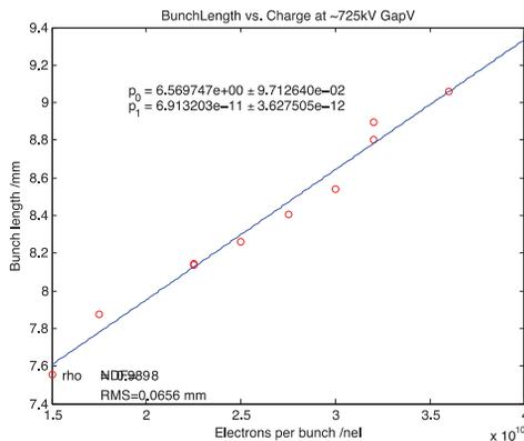
Figure 4: Bunch length in mm vs. ring current as measured in the NRTL in e- per bunch.
