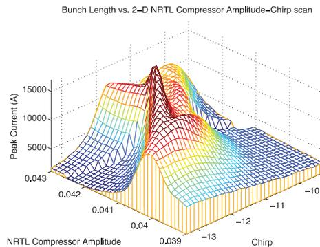
Figure 6: Simulated peak current from LiTrack in the FACET experimental area for 6mm long NDR bunches as a function of NRTL compressor amplitude and “staggered\_chirp” setting.
