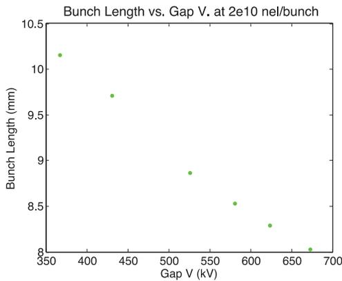
Figure 3: Bunch length in mm vs. NDR gap voltage in kV.
