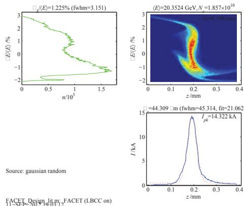
Figure 9: Simulated bunch profile from LiTrack in the FACET experimental area for 8mm long NDR bunches.
