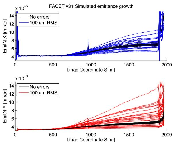
Figure 5: Effects of RF structure misalignment on horizontal (top) and vertical (bottom) normalized emittance growth in FACET. 30 beams are tracked to the dump, with random transverse offsets (0.1 mm RMS) applied to each end of the S-band accelerating structure. Results for perfectly aligned structures are plotted in black.
