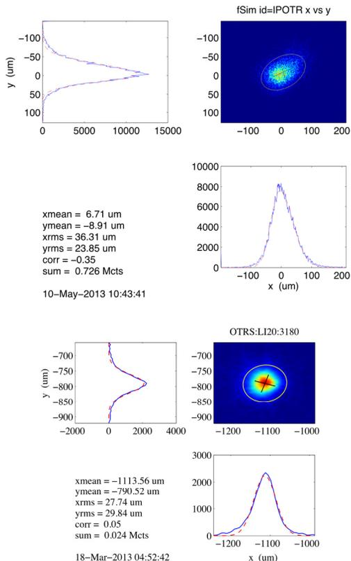
Figure 3: Simulated (top) and real (bottom) transverse beam profiles measured at the plasma IP diagnostic OTR.
