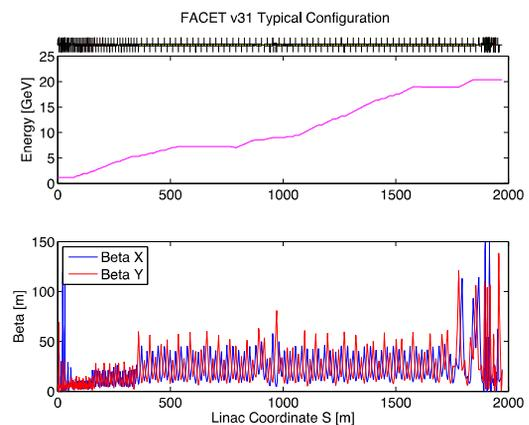
Figure 2: fSim model snapshot of accelerator state. The momentum profile (top) and Twiss functions (bottom) are calculated from control system readbacks of magnet excitation, RF amplitudes, etc.
