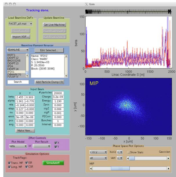
Figure 1: fSim interface with z-plot of Twiss functions and simulated beam profile at the FACET plasma IP.
