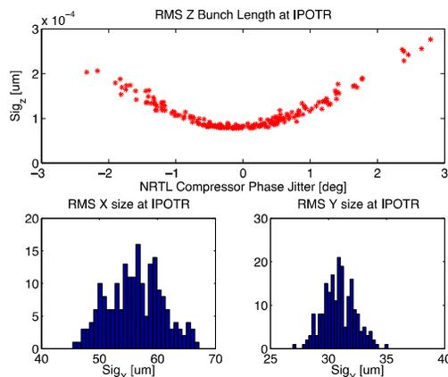
Figure 4: 200 tracked beams, each with 1 degree RMS random phase jitter applied to linac klystrons. Top: RMS bunch length at plasma IP is most sensitive to jitter in the NRTL compressor klystron. Bottom: Distribution of transverse beam sizes.
