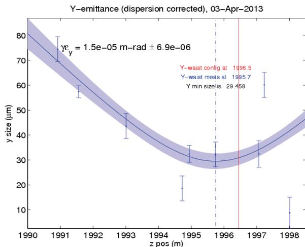
Figure 9: Vertical beam size measurements in the FACET experimental area giving an emittance of 1.5 E-5 m-rad.
