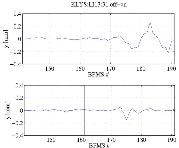
Figure 5: Vertical difference orbit for klystron 13-3 off-on shows the generation of a big dispersion wave at BPMS #175 (Li14 901), top. While a -3 mm orbit bump there cancels the downstream wave considerably, bottom.
