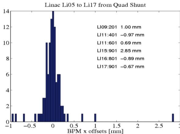
Figure 2: Distribution of the horizontal BPM to quadrupole offsets from quad-shunting.
