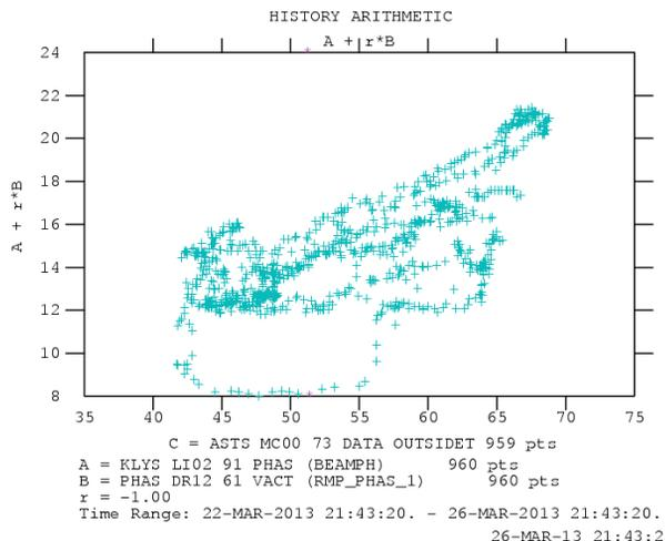
Figure 10: The variation of the linac injection phase minus measured beam phase versus the outside temperature.
