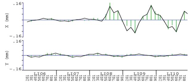
Figure 6: Corrector hysteresis: XCOR LI08 402 all up and back (orbit), minus all down and back up (reference). The 3.65  $\mu$ rad kick in x correspond to 1.5 kG-mm or 4.4% of the maximum corrector strength.
