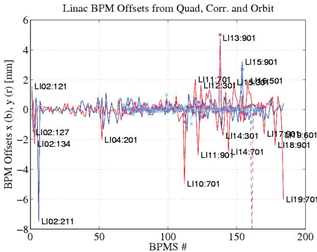
Figure 4: BPM offset along the linac. Stronger correctors seen as apparent BPM offsets show up in the second half.
