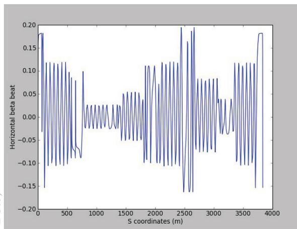
Figure 5: Introduced horizontal beta-beat with controlling required strength change.
