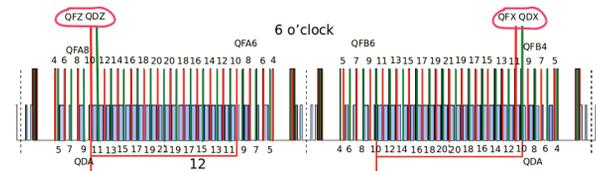
Figure 1: Beamline around IP6, quadrupole QFZ, QDZ, QFX and QDX are used for matching in  $\pi$ -doublet solution.
