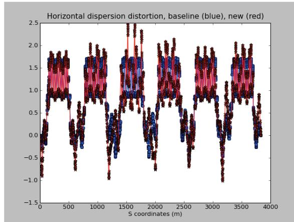
Figure 4: Baseline and new horizontal dispersion functions in QF8+QF9 solution.
