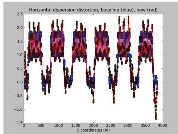
Figure 7: Baseline and new horizontal dispersion functions with controlling required strength change.
