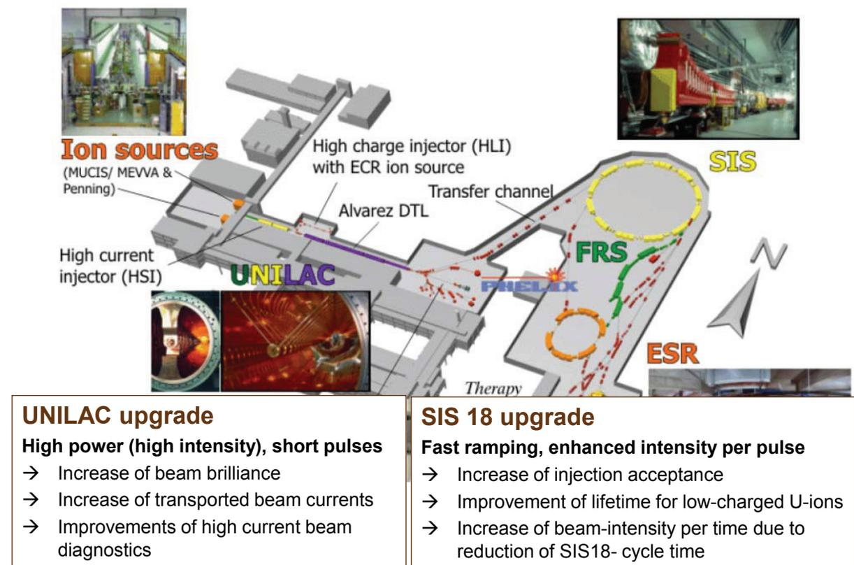
Figure 2: Overview of the GSI accelerator facility and the upgrade program of the UNILAC and the SIS18.
