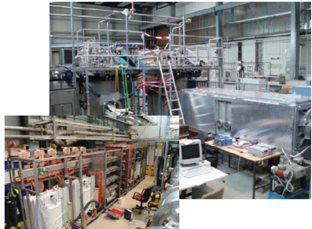
Figure 4: Magnet test facility at GSI including the new 20 kA pulse power supply.
