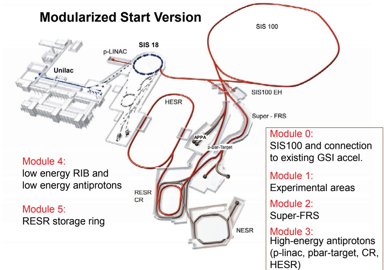
Figure 1: Overview of the FAIR accelerator facility and the modules 0-5 of the different accelerator and experiment sections. Modules 0-3 represent the modularized start version, which will be realized.
