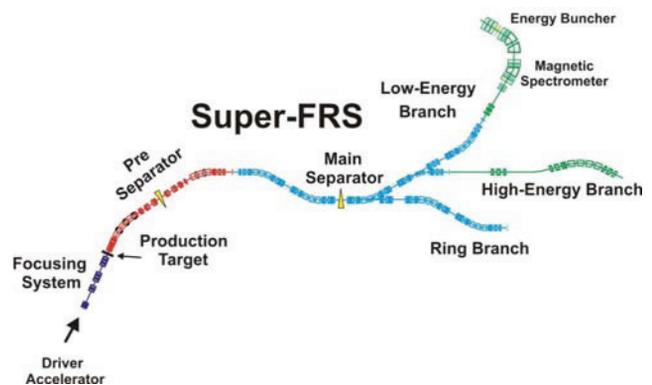
Figure 3: Lay-out of the Super-FRS of the FAIR facility.
