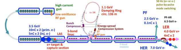
Figure 8: Upgrade of the injector Linac and a new positron damping ring.
