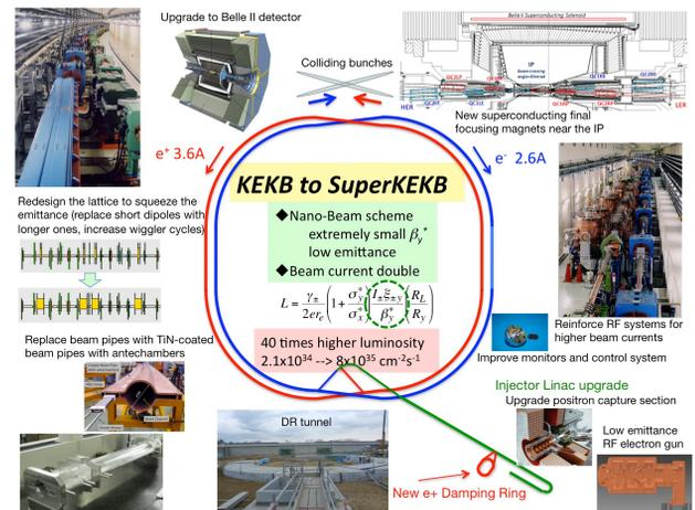
Figure 1: Layout and scheme for SuperKEKB.
