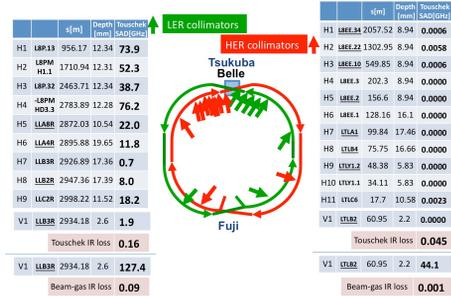
Figure 3: Optimized layout of the collimators [12].
