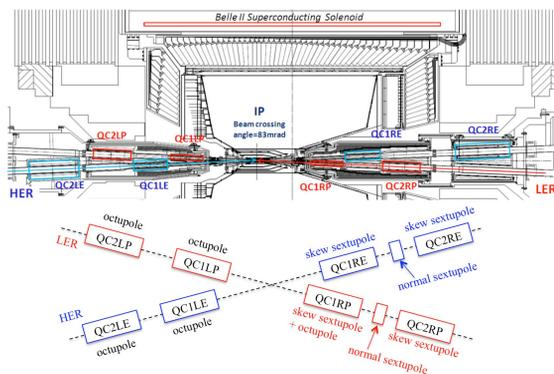
Figure 2: Schematic drawing of the final focus system of SuperKEKB (upper) and layout of sextupole and octupole corrector coils (lower).
