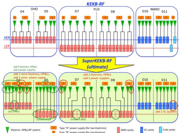
Figure 7: Rearrangement and reinforcement of the RF system.
