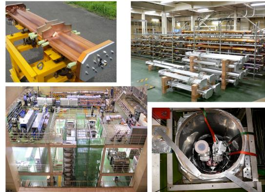
Figure 5: Copper and aluminum antechamber-type beam pipes (upper). Vacuum work deck, and TiN coating and baking facilities (lower).
