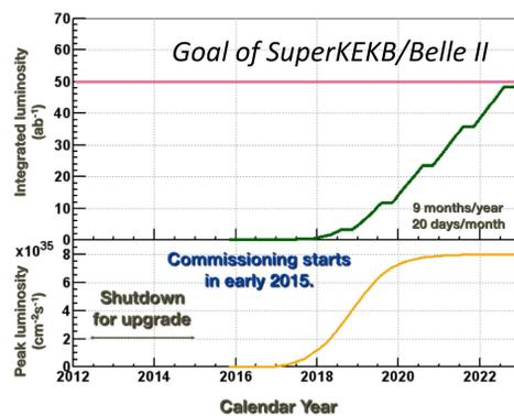
Figure 9: Luminosity projection of SuperKEKB.
