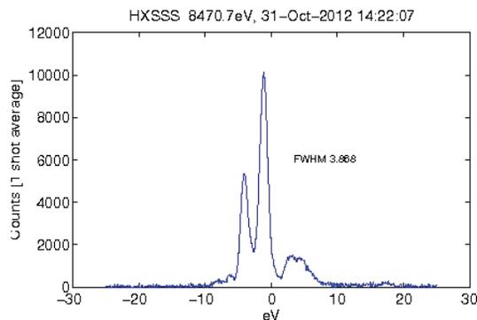
Figure 6: An iSASE FEL spectrum with undulator in Fig. 5.
