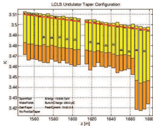
Figure 5: Undulator setup for iSASE experiment at LCLS.
