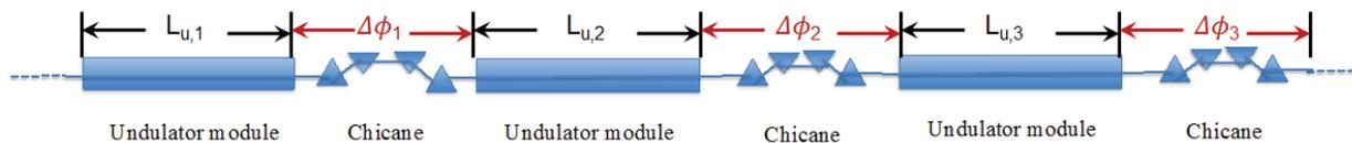
Figure 1: Illustration of implementing phase shifter (e.g., a magnetic chicane) between undulator modules.
