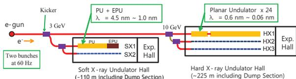
Figure 3: Layout of hard X-ray and Soft X-ray FEL line.
