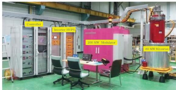
Figure 4: A proto-type of klystron modulator.
