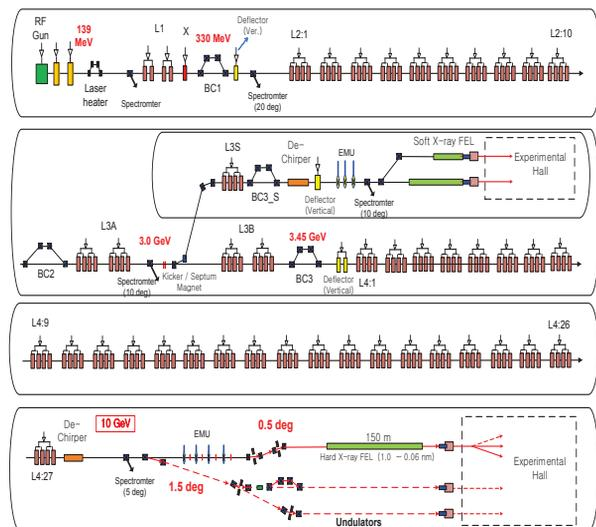
Figure 2: Schematic layout of the 3-BC lattice of PAL-XFEL.
