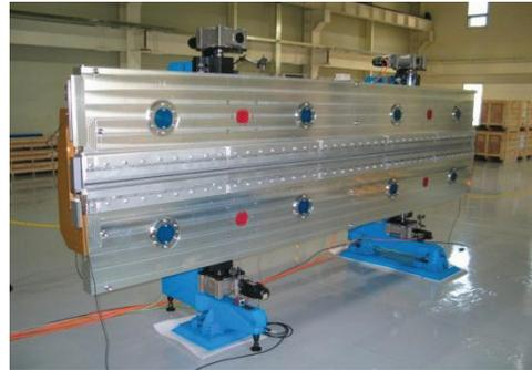
Figure 7: A proto-type of undulator.
