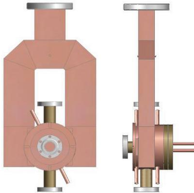
Figure 6: Photocathode RF-gun.
