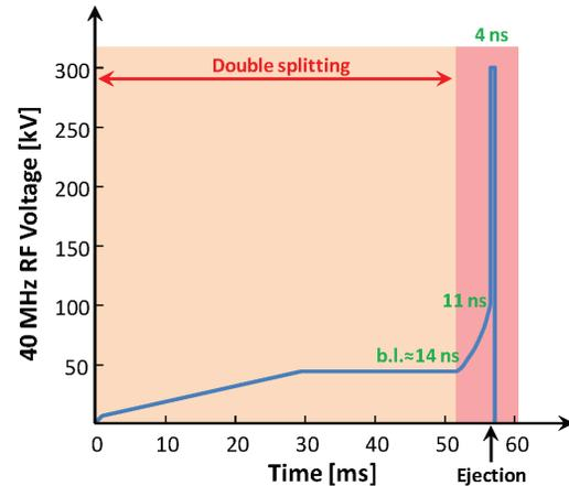
Figure 1: RF voltage (40 MHz) program during the last stages of the cycle for the production of the LHC type beams. The total ( $4\sigma$ ) bunch length is reported in green.
