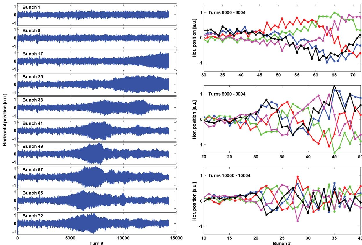
Figure 2: (Left) Evolution of the horizontal centroid position for selected bunches along the bunch train ( $t=0$  roughly corresponds to the beginning of the bunch shortening); (Right) bunch by bunch position for five consecutive turns, at different moments during the store (the horizontal scale is chosen in order to better visualize the unstable bunches).
