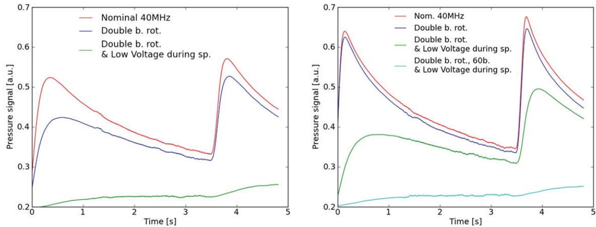
Figure 3: Pressure measured with two consecutive LHC type cycles (the beam is extracted at  $t=0$  and  $t=3.6$  s) for different RF manipulations. Comparison between two different bunch intensities:  $\sim 1.25 \times 10^{11}$  ppb on the left and  $\sim 1.45 \times 10^{11}$  ppb on the right.
