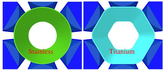
Figure 13: Beam pipes of sextupole.
