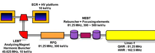
Figure 1: Schematic layout of the driver linac.
