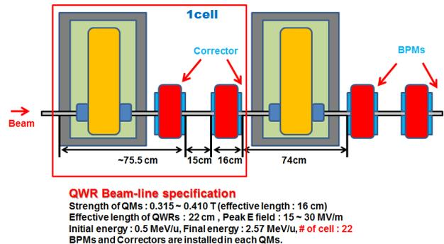
Figure 2: Schematic layout of two cell of the low energy linac.
