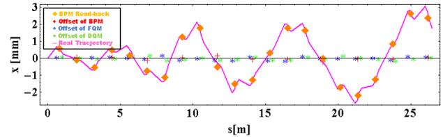
Figure 4: Beam orbit in the low energy linac with error of the elements.
