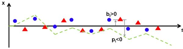
Figure 3: Scheme of the kick due to the alignment error of the elements.
