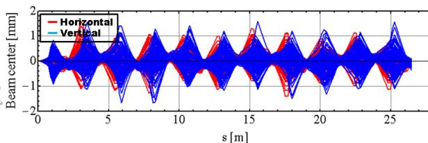
Figure 7: Scheme of the kick due to the alignment error of the elements.
