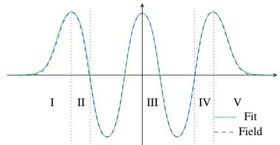
Figure 2: Simulated field, matched field and the sections of the matched field. The input/output exponential decay (I/IV), input/output sinusoidal (II/IV), and inner cells (III).
