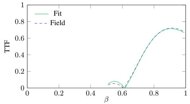
Figure 3: TTF calculated for a range of  $\beta$ s using the field from RF simulations and the fitted field.
