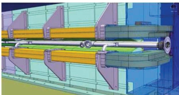
Figure 1: Location of the flanges for the new electron cloud monitors within a main magnet (Courtesy of T. Capelli).
