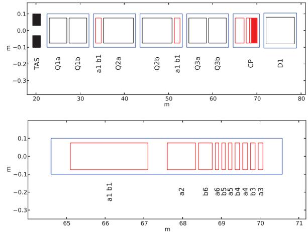
Figure 1: Upper: Sketch of the latest HL-LHC IT and D1 layout with associated correctors [3]. Lower: zoom of the triplet corrector package. The horizontal scale indicates the distance to the IP.
