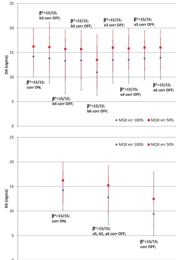
Figure 3: Impact of the absence of one corrector on the dynamic aperture (upper). Impact of the absence of groups of correctors on the dynamic aperture (lower). The blue series refers to simulations performed with the full multipoles from Table 1, while the red one refers to simulations performed with 50 % of the multipoles.
