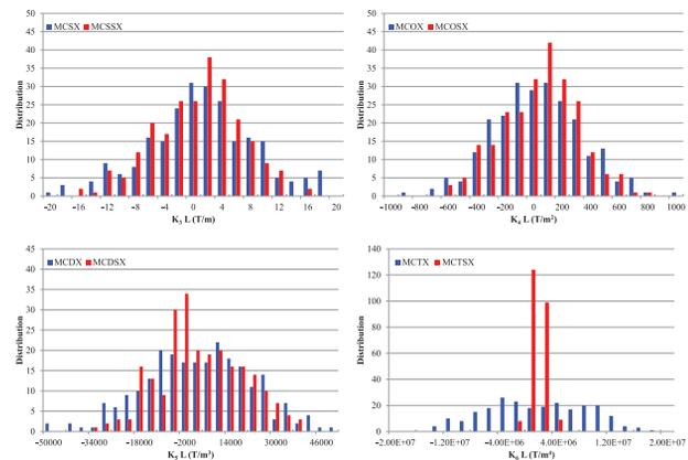
Figure 2: Distribution of the strength of the non-linear correctors:  $a_3, b_3$  (upper left);  $a_4, b_4$  (upper right);  $a_5, b_5$  (lower left);  $a_6, b_6$  (lower right).
