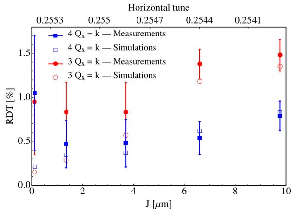
Figure 6: RDT vs.  $J$  for sextupolar and octupolar resonances in the case of the standard PS configuration at 14 GeV/c with additional single sextupole magnets turned on. Both measurements and simulations results are shown for the sake of comparison. The measured tune is reported in the second horizontal scale.
