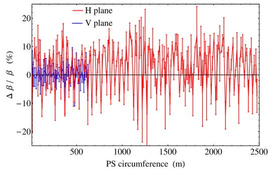
Figure 2: Measured  $\beta$ -beating for a bunch kicked inside a stable island generated at 14 GeV/c (The PS circumference is  $2\pi 100$  m long).
