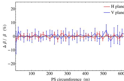
Figure 1: Measured  $\beta$ -beating for the PS ring at 14 GeV/c.
