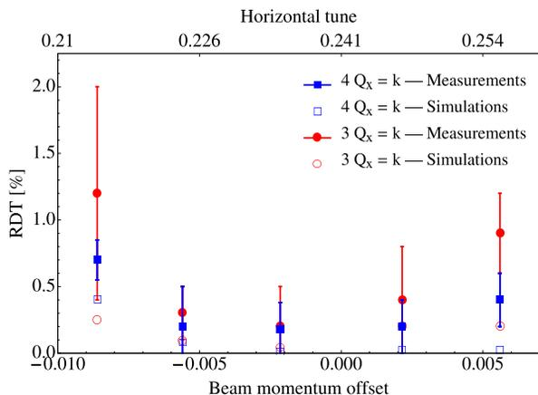
Figure 5: RDT vs. beam momentum offset for sextupolar and octupolar resonances for the standard PS configuration at 14 GeV/c. Both measurements and simulations results are shown for the sake of comparison. The measured tune is reported in the second horizontal scale.
