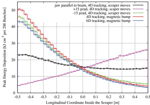
Figure 3: Longitudinal pattern of the peak energy deposition in the LIU SPS scraper, for different simulation settings. Error bars indicate to statistical errors.
