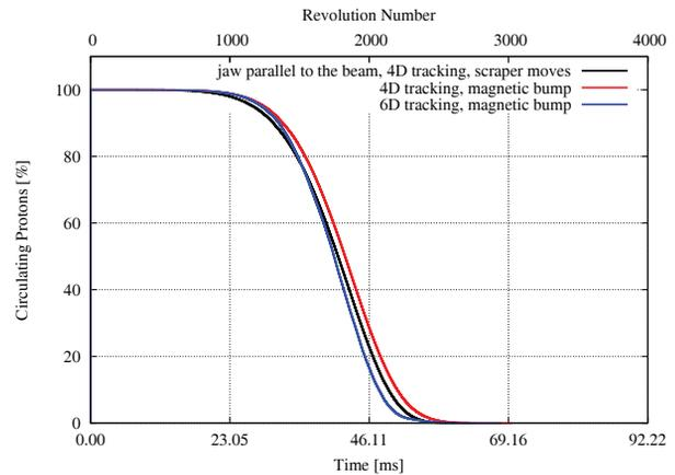
Figure 4: Evolution in the number of beam particles with time, from the beginning of the simulation. The equivalent turn numbers are indicated as well.
