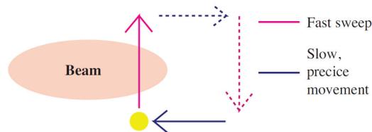
Figure 1: Schematic view [5] of the movement of the SPS scraper jaw during operation: tails outside a desired amplitude are cut off by means of a fast movement through the beam, starting from the parking position (marked by the yellow spot). Only the horizontal scraper is shown.
