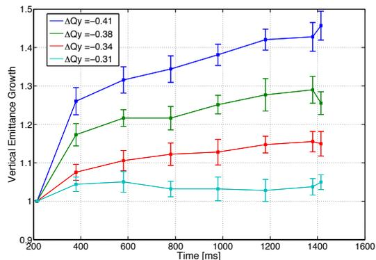
Figure 6: Time evolution of the vertical emittance blow-up for four different space charge maximum detuning.
