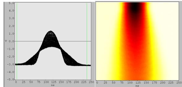
Figure 4: Longitudinal beam profiles during an adiabatic bunch compression.
