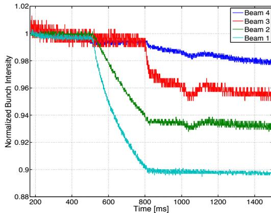
Figure 3: Losses during crossing  $4Q_y = 25$  resonance.
