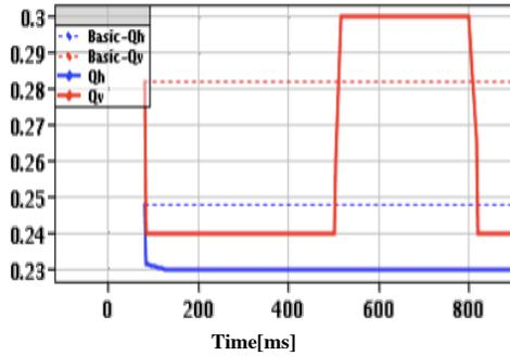
Figure 2: Horizontal and Vertical programmed tunes (continuous lines) and nominal horizontal and vertical tunes (dashed lines) along the measurement magnetic plateau.
