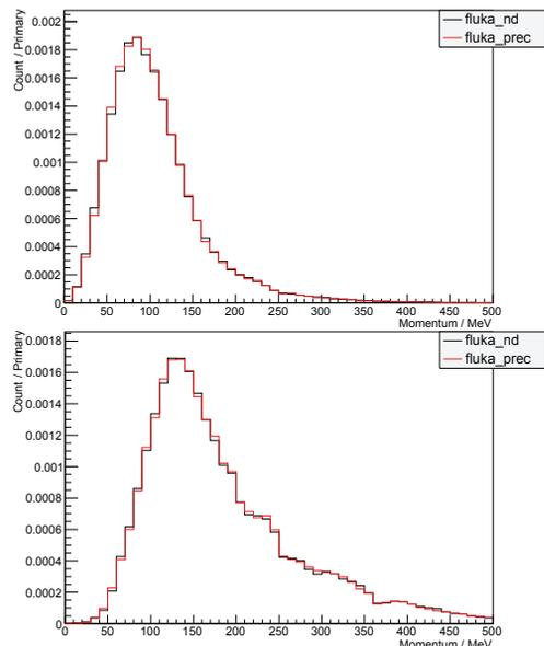
Figure 3: Momentum distribution of muons (top) and pions (bottom) at the entrance of the muon torus produced by the FLUKA default (fluka\_nd) and precision (fluka\_prec) models. The vertical scale is normalised to the number of primary protons used in the simulation.
