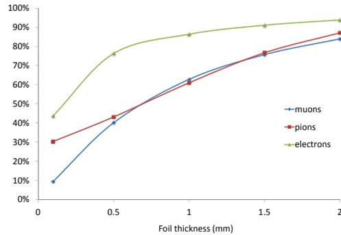
Figure 8: Percentage of pions, muons and electrons stopped by the tungsten absorber for different thicknesses.
