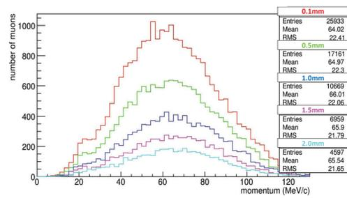
Figure 7: Momentum of muons after the tungsten absorber for different thicknesses.
