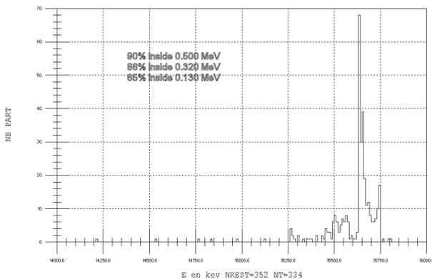
Figure 9: Energy histogram at the buncher exit.
