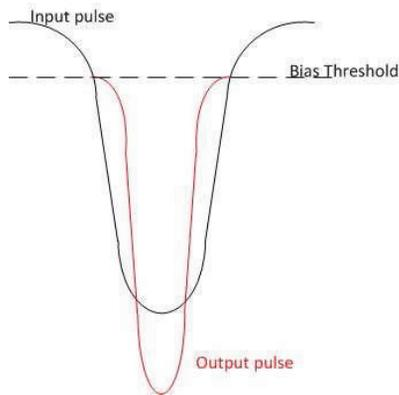
The final width of the Single Pulse Mode electron beam delivered is close to 500 ps at the output electron gun.
