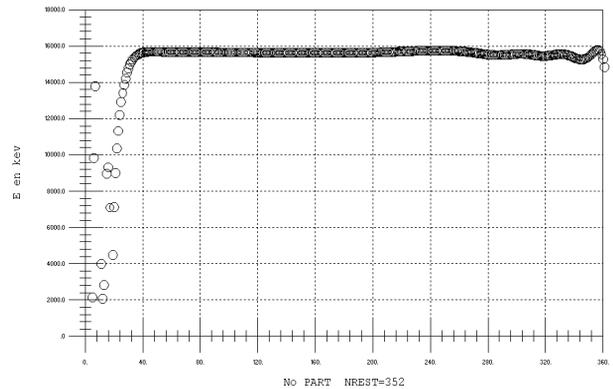
Figure 8: Energy at the buncher exit.
