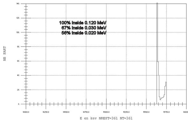
Figure 12: Energy histogram at buncher exit for 500 ps.
