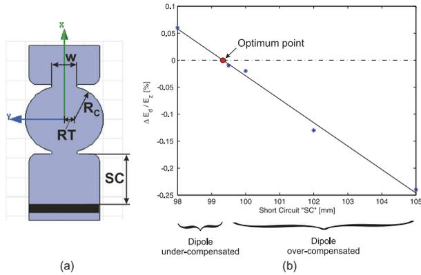
Figure 2: Racetrack geometry applied to the single feed coupler with movable short-circuit (a) and plot of the dipole component for a small variation of the parameter “SC” (b).
