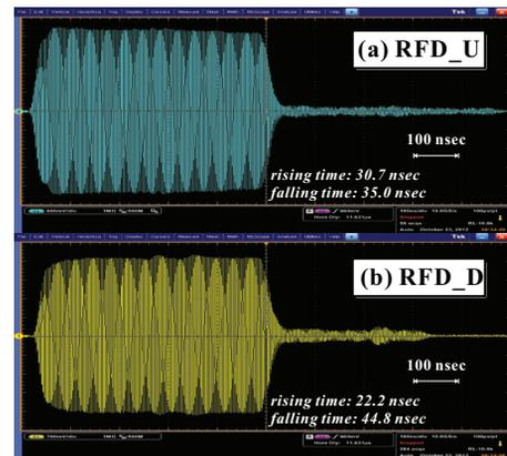
Figure 4: RF pickup signals of (a) RFD\_U and (b) RFD\_D in the parallel-connected system. The ringing on the RF falling of RFDs was suppressed in comparison with Fig. 1.
