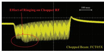
Figure 2: Chopped beam (FCT05) in the series-connected system. The dent on the beam head was observed. It was thought as the cause of the ringing on the period of the RF falling.
