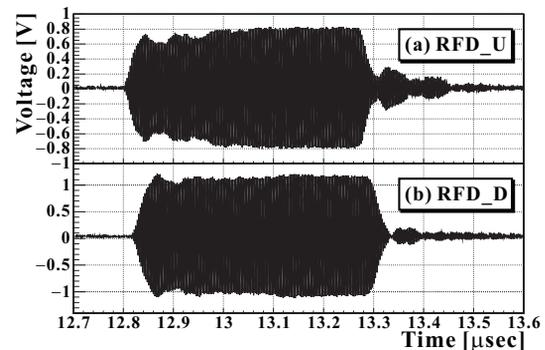
Figure 1: RF pickup signals of (a) RFD\_U and (b) RFD\_D in the series-connected system. The large and long ringing on the RF falling of RFDs, especially RFD\_U, was observed.
