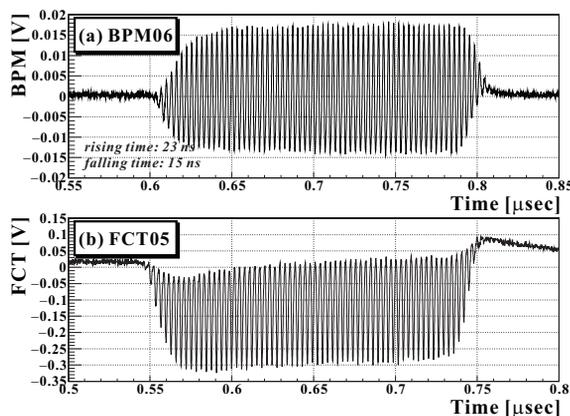
Figure 7: Chopped beam in the system of the parallel-connected system with (a) BPM06 and (b) FCT05. It could be confirmed that the effect of the ringing decreased.
