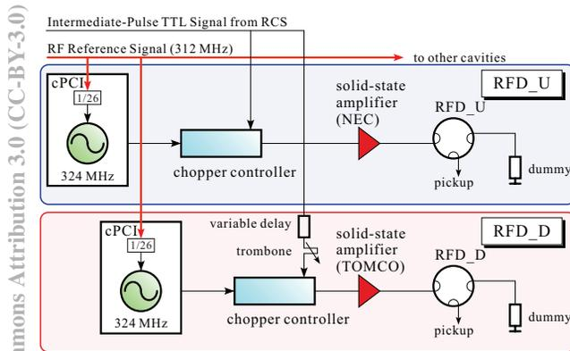
Figure 3: Schematic diagram of the parallel-connected system. There are two RF sources by each RFD.
