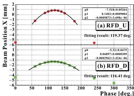
Figure 5: Results of the phase tuning for (a) RFD\_U and (b) RFD\_D. Each phase was adjusted to be the largest deflecting angle.
