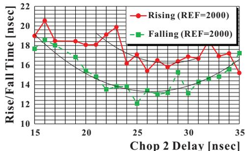
Figure 6: Results of the relative timing tuning. The red circles and the green squares show that for the rising and the falling, respectively.
