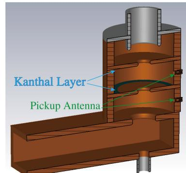
Figure 1: The cross section of the lossy cavity.
