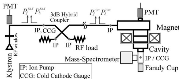
Figure 4: High power test configuration.
