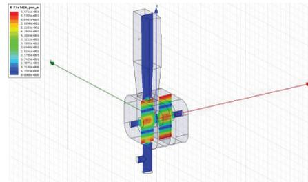
Figure 4: Magnetic field distribution in 2 cell rf-deflector cavity by HFSS.
