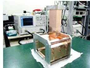
Figure 8: Photo of 2 cell rf-deflector cavity
