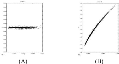
Figure 7: Bunch profile of TY plane (A): deflector is off, (B): deflected bunch at the zero-crossing phase
