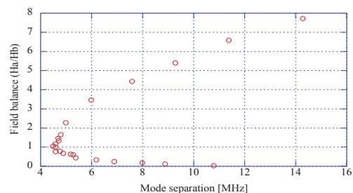
Figure 5: Field balance as a function of mode separation
