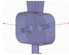
Figure 3: Single-cell structure of the rf-deflector.
