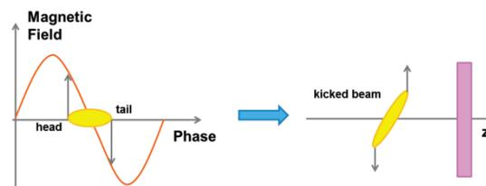
Figure 2: Effect of the transverse magnetic field generated by rf-deflector cavity.
