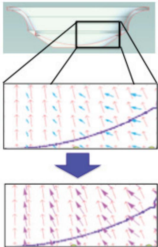
Figure 8: The cathode outline of the klystron used in the power test (top). The blue arrows are the calculated magnetic field on the cathode at the first power test. The red arrows are the calculated magnetic field generated by electromagnet (middle). The purple arrows are the calculated magnetic field on the cathode after the Fe oil tank is introduced (bottom).
