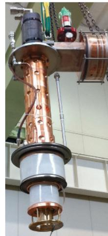
Figure 4: The klystron used for power test (Toshiba E37501).
