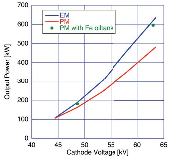
Figure 7: The result of the klystron power test.
