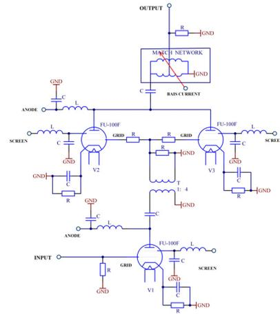
Figure 4: Schematic circuit diagram of FB amplifier
