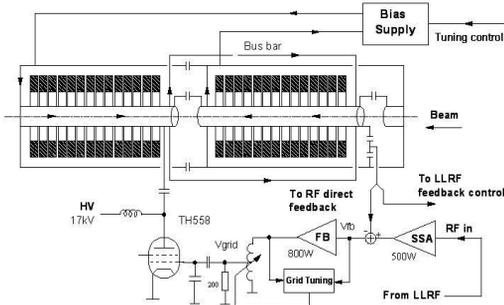
Figure 3: CSNS RCS RF system simplified schematic
