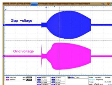
Figure 8: Waveforms of the cavity gap and tube grid operated in sweeping mode with repetition rate of 25Hz.
