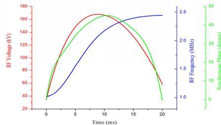
Figure 1: RCS RF voltage, synchronous phase and RF frequency patterns during accelerating time of 20ms.
