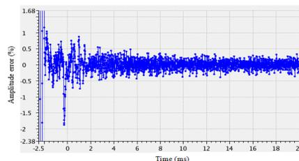
Figure 9: Cavity gap voltage amplitude error within a cycle of 20ms.
