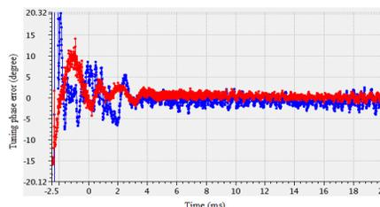
Figure 10: Cavity detuning angle (blue) and Grid tuning error (red) within a cycle of 20ms
