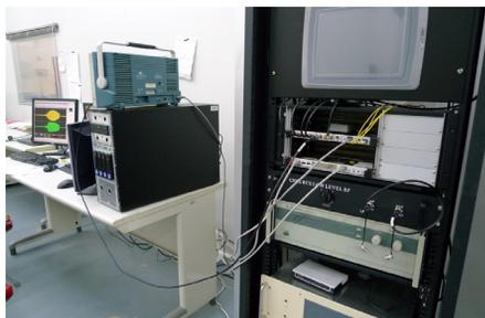
Figure 7: Digital LLRF control system prototype
