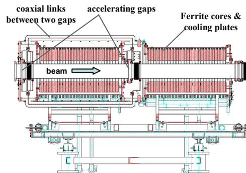
Figure 2: CSNS RCS RF cavity
