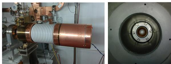
Figure 4: Gun test stand (left) and cathode grid assembly installation (right).
