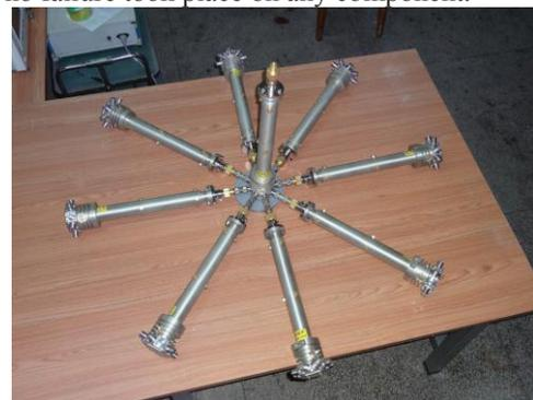
Figure 6: 1-64 power splitting system.
