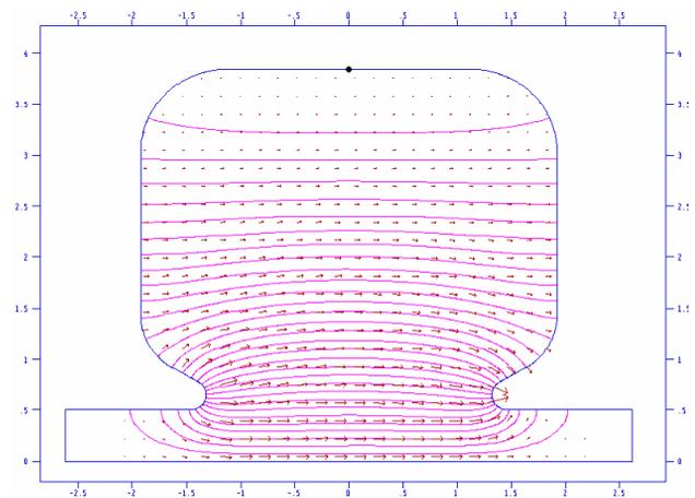
Figure 1: Cavity shape and field distribution of main accelerator.
