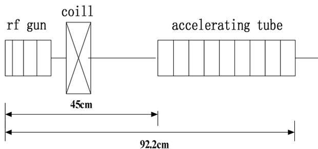
Figure 3: Simulation model of beam dynamics.
