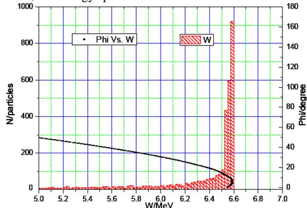
Figure 4: Energy density distribution and energy vs. phase distribution at the exit of main accelerator.
