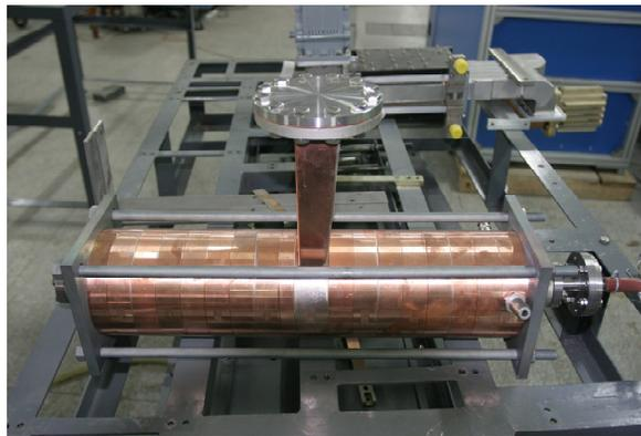
Figure 5: Photo of main accelerating tube after welding.
