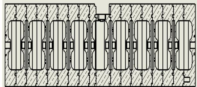
Figure 2: Cutaway view of the accelerating tube.
