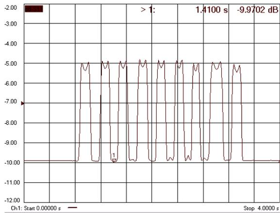
Figure 6: The measured result of field distribution of the accelerating tube.
