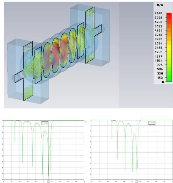
Figure 3: Simulation and S11 of two matching coupler.
