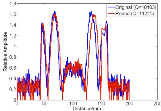
Figure 2: R/Q results of two types cavity on  $4\pi/5$ .
