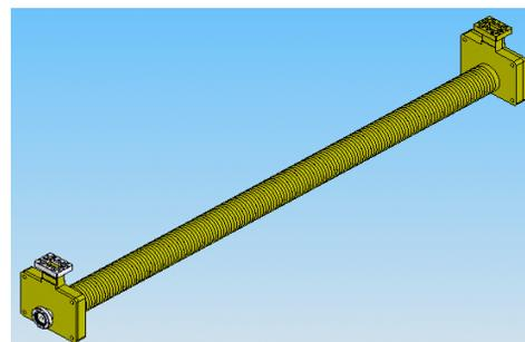
Figure 5: 3D design of new C-band accelerating structure.
