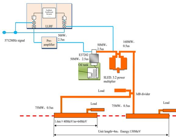
Figure 6: C-band RF system scheme for SXFEL.
