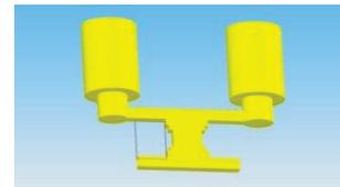
Figure 2: Schematic of the SLED type pulse compression.
