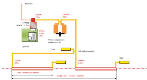
Figure 1: The schematic diagram of the R&D microwave unit.
