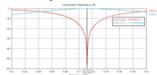
Figure 12: Simulated S-parameter of the mode converter.
