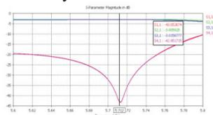
Figure 10: Simulated S-parameter of the 3-db coupler.
