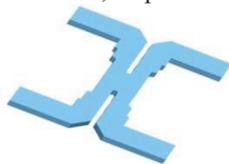
Figure 9: Schematic drawing of the 3-db coupler hybrid.
