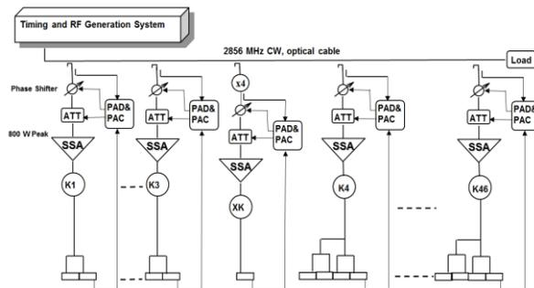
Figure 1: Microwave system for PxFEL.
