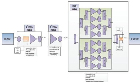
Figure 2: Block diagram of SSA.
