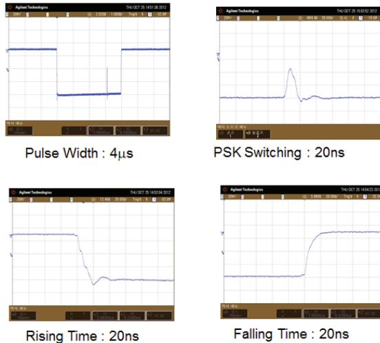
Figure 6: Waveform of SSA Output.
