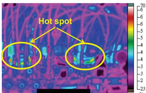
Figure 7: The thermal spot happened during high power RF vacuum condition.
