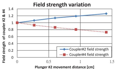
Figure 6: At balance field situation, the coupled field strength power would have the same amplitude variation but opposite direction at cell #2 and #4 by moving just one plunger at cell #2.
