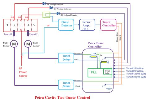
Figure 10: The automatic in-situ balance controller for real time separately control two plungers for balance field distribution with calibrated couplers on each cell.
