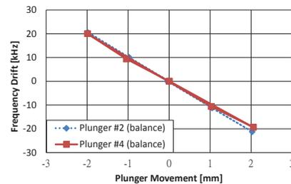
Figure 5: The frequency drift caused by the same movement of plungers in balance field distribution.
