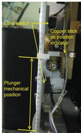
Figure 2: The ruler for plunger position monitor.
