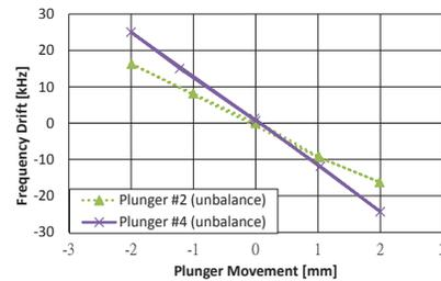
Figure 4: The frequency drift caused by the same movement of plungers in unbalance field distribution.
