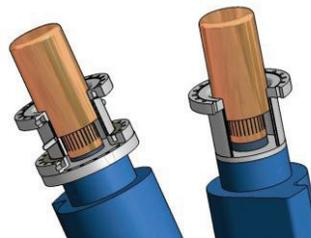
Figure 8: The plunger modification with cooling water channel added for better vacuum during RF processing (left figure) and original design (right figure).
