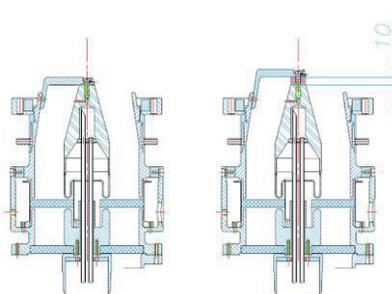
Figure 9: The coupling coefficient changing from 1.7 to 2.2 by extending the coupling length by 10mm.
