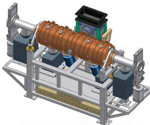
Figure 1: Layout of 5-cell Petra Cavity with All its accessories.
