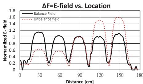
Figure 3: The balance and unbalance field distribution by control the position of two plungers.
