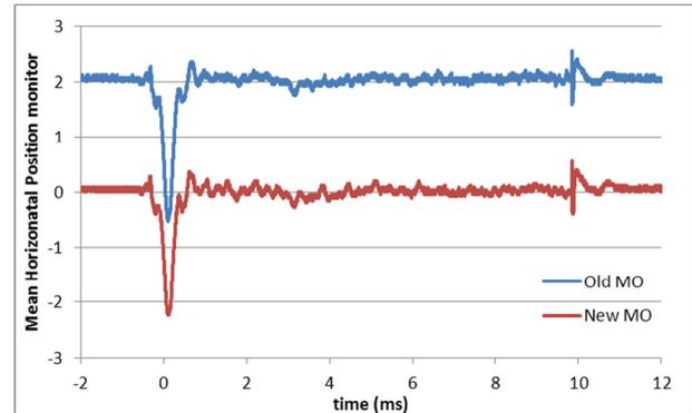
Figure 4: Mean horizontal beam position signal for the Old MO (2V offset) compared with the new FPGA MO with improved input signal buffering.
