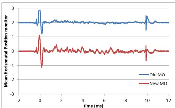
Figure 3: Mean horizontal beam position signal for the Old MO (2V offset) compared with the new FPGA MO.
