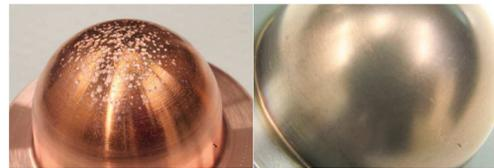
Figure 3: Photos of a Cu (left) and Be (right) button after high-power RF testing.  $\mu\text{m}$ -scale damage is present on the Be button surface, but is not visible to the naked eye. Damage on the Cu button is mm-scale.
