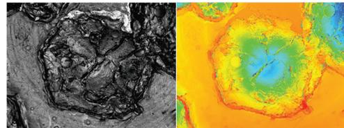
Figure 4: Typical LCSM images of damage on a Cu button. The right-hand image is a false-color map containing height information. Warm colors (red, orange) are closer to the camera than cool colors (blue, green). This crater has a maximum depth of  $73.79 \pm 0.01 \mu\text{m}$ , an effective diameter at the rim of  $430 \mu\text{m}$ , and a volume of  $(2.592 \pm 0.002) \times 10^6 \mu\text{m}^3$ .
