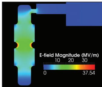
Figure 2: Simulation of the electric field inside the 805 MHz pillbox cavity, using SLAC's ACE3P code suite [8].
