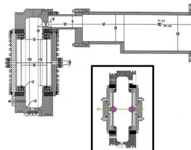
Figure 1: Schematic of the 805 MHz pillbox cavity. The gap length is 81 mm and the radius is 158 mm. The inset shows the cavity with buttons installed (purple) and the direction of the applied magnetic field (green).
