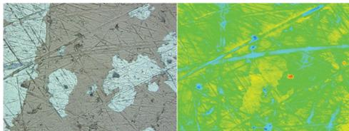
Figure 5: LCSM images of damage on a Be button. Damage sites may be concave (as for Cu damage) or convex. X-ray diffractometry reveals the light patches as bare Be, after the TiN film was vaporized during breakdown events. Note that TiN is not missing in the vicinity of every damage site.
