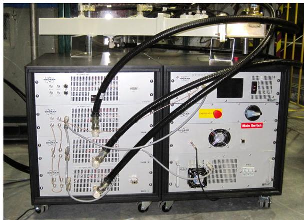
Figure 1: The 1.3GHz, 5kW, Solid State Amplifier. The three power modules are installed on the left side, the right side contains the power transformer and the status screen is located on the top right panel.
