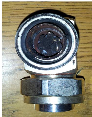
Figure 2: The Damaged Cable Connector.
