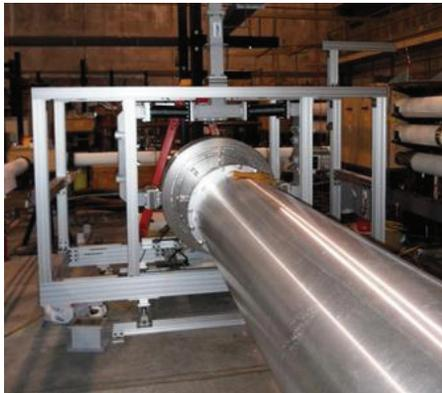
Figure 1: Photograph of the test setup of the nitrogen filled, aluminium, circular pipe in which power enters from the top via WR650 waveguide and is split with a magic T to feed the mode launcher.
