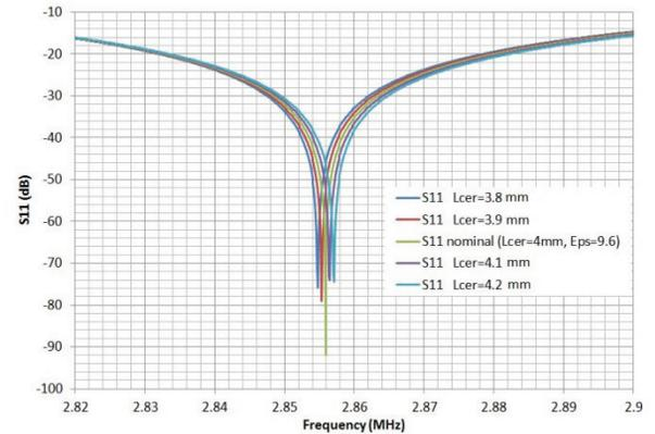
Figure 2: Reflection vs. frequency for varying ceramic thicknesses.
