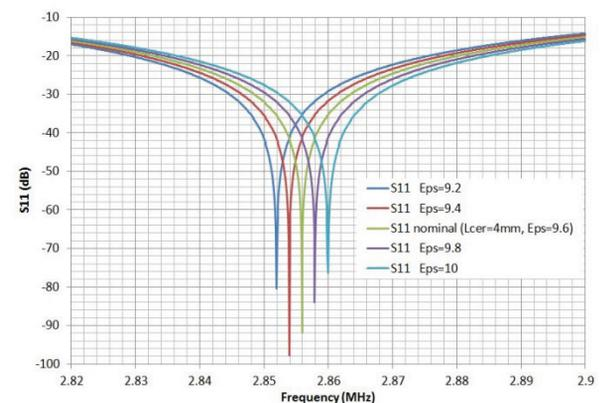
Figure 3: Reflection vs. frequency for varying ceramic permittivity.
