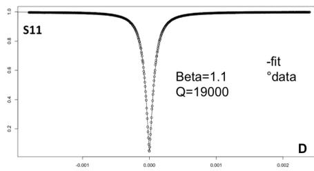
Figure 6: Measured Reflection coefficient (S11).
