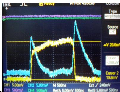
Figure 9: Power waveforms from oscilloscope. Forward (yellow) and reflected power (blue).
