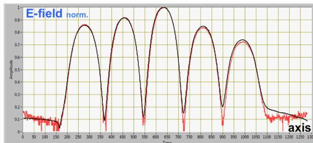
Figure 7: Axial electric field profile (bead-pull).
