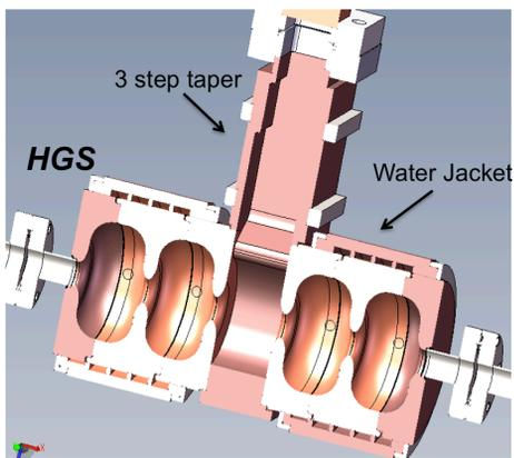
Figure 3: 3D mechanical model (SolidWorks) of the 5-cell HGS structure.
