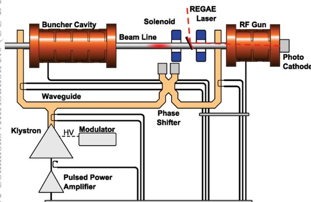
Figure 1: Overview of the RF system installed at REGAE
