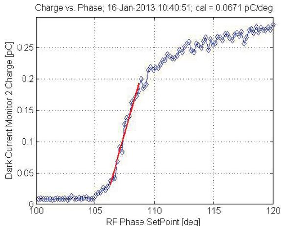
Figure 4: Charge measured versus RF gun phase during a phase scan. The linear fit (red) shows the region with the highest sensitivity (0.0671 pC/deg).
