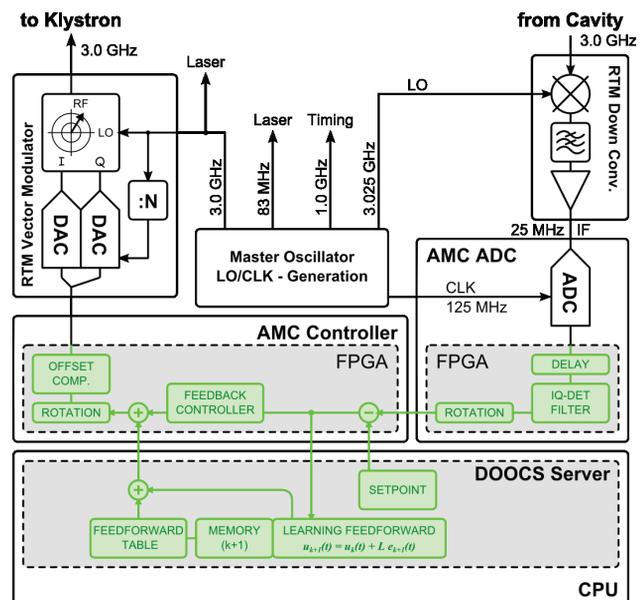
Figure 2: Overview of the LLRF system at REGAE
